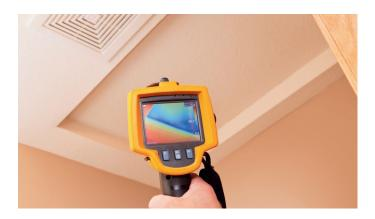
Walls: infrared testing showed thermal bridging (heat loss) at studs due to lack of continuous exterior insulation, degrading R value to below code levels; recommendation: add exterior insulation.
